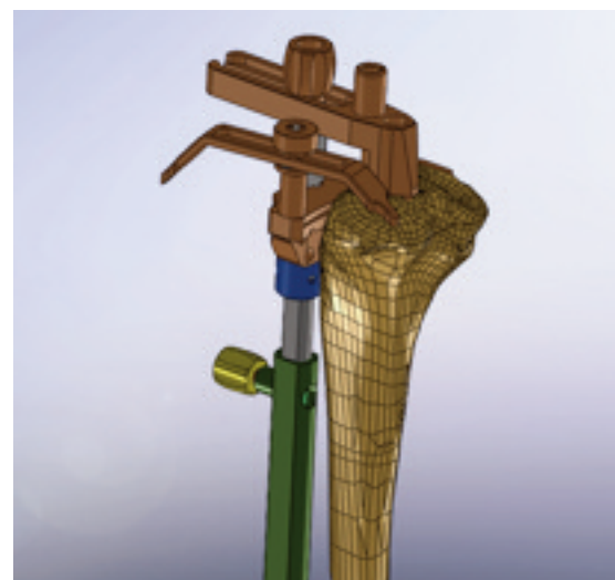
The stylus tip marked '10mm' indicates a 10 mm thick bone resection.
